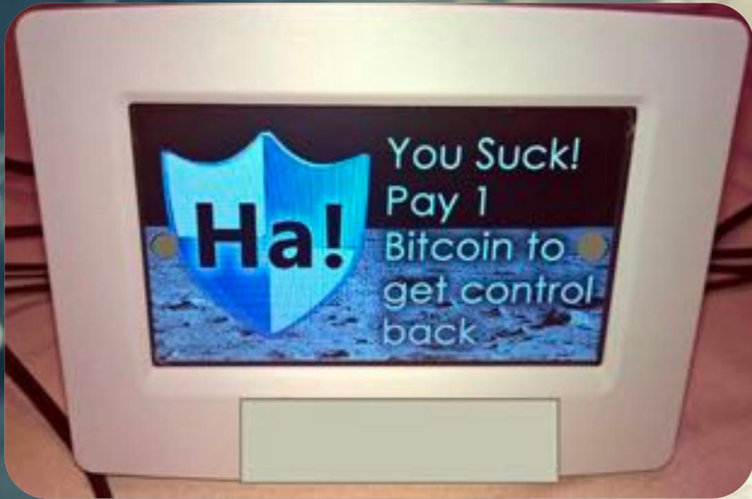
Everything in the thermostat runs with **root** privileges. “**We got command injection by the SD card**, so it was a local attack,” Tierney explained. “With root, you can set off alarm (and set the frequency very high) and can heat and cool at the same time.”
