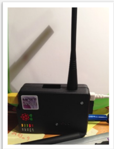
POC Raspberry PI with custom made shield for radio transmissions
